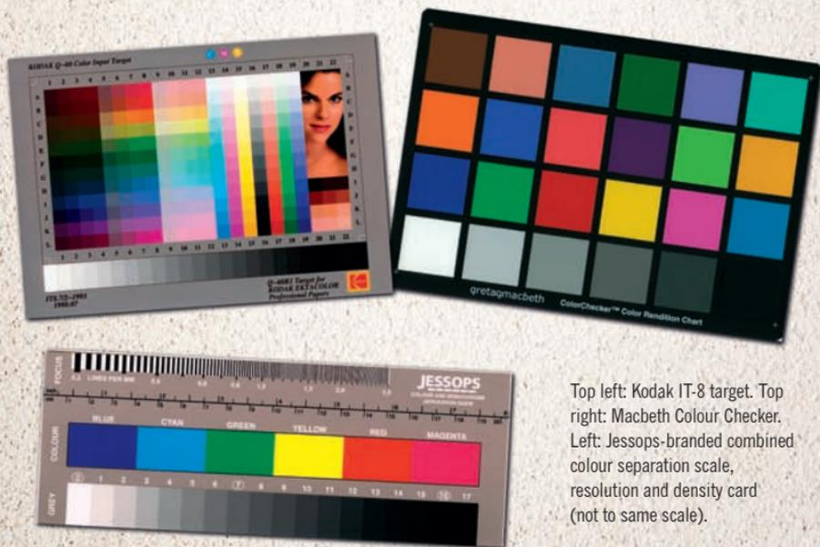
Top left: Kodak IT-8 target. Top right: Macbeth Colour Checker. Left: Jessops-branded combined colour separation scale, resolution and density card (not to same scale).
