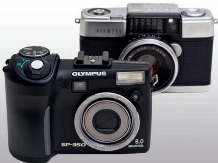
An 8 MegaPixel SP350 digital compact zoom camera (2005) features a tiny zooming optical viewfinder, despite having a large rear LCD screen. Shown behind is a 35mm half-frame classic (1962), the Pen D, which relied solely on the optical viewfinder with parallax lines for framing.
