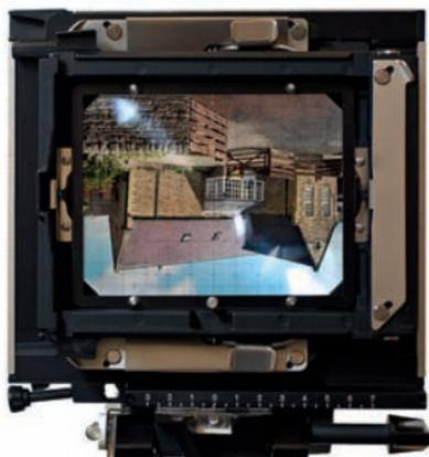
This image of the screen on a 5x4 camera has been enhanced to show how the image appears under the cloth.
