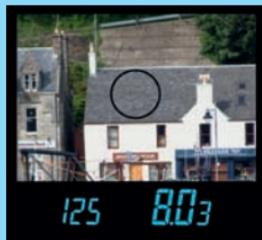
Spot readings can be taken from a mid-tone in the image or an average exposure calculated from readings of shadows and highlights. Spot meters are favoured by zone system workers for their precision in measuring small areas of tone.
