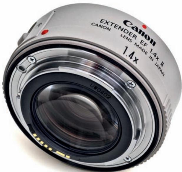
TELE-CONVERTERS ARE SUPPLEMENTARY LENS SYSTEMS FITTED BETWEEN THE LENS AND CAMERA BODY TO EXTEND THE EFFECT OF TELEPHOTO LENSES. THEY COME IN A RANGE OF POWERS:  $\times 1.4$ ;  $\times 1.7$  AND  $\times 2$  ARE COMMONLY OFFERED. A  $\times 2$  TELE-CONVERTER WILL DOUBLE THE FOCAL LENGTH OF A LENS, MAKING A 600MM LENS A 1,200MM OPTIC, WHEREAS A  $\times 1.4$  WOULD GIVE IT AN 840MM FOCAL LENGTH. SADLY, A  $\times 2$  CONVERTER WILL ALSO HALVE THE APERTURE, MAKING A 600MM F/4 LENS A 1,200MM F/8.
