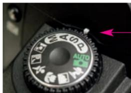
The mode is marked S (Shutter) or TV (Time value) on the camera mode dial or menu.
