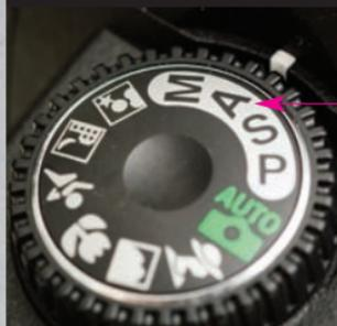
The mode is marked A (aperture) or AV (aperture value) on the camera mode dial or menu. Aperture priority is ideal for portraiture or some garden photography, when a wide aperture is chosen to keep the background out of sharp focus.
