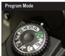
Both Program and Auto Exposure modes set shutter speed and aperture automatically; Auto mode will also use the built-in camera flash in low light situations in preference to a long shutter speed or wide aperture.
